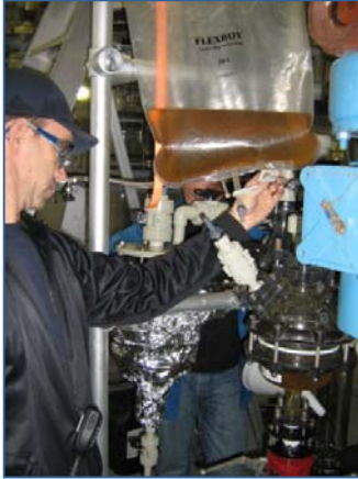
Figure 2: Addition of inoculum to the growth reactor
